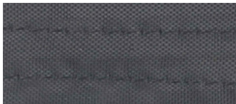
96 hours at 120°C on the heating cable: no color change, no insulation melting, no change in characteristics
