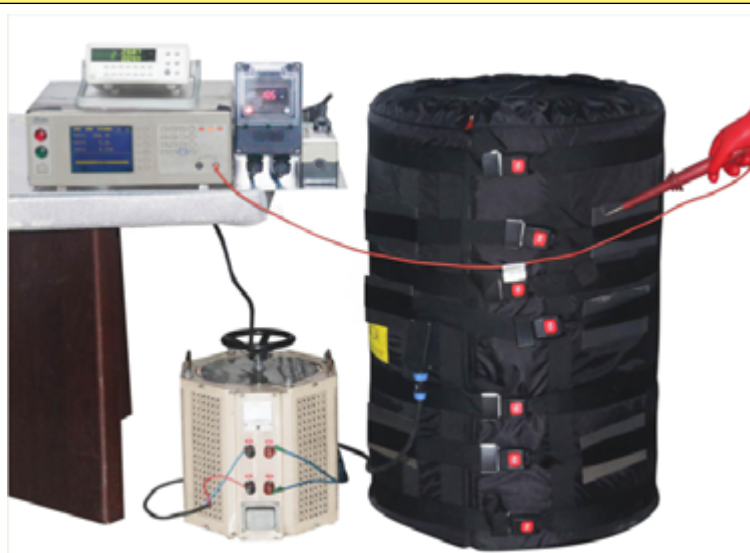
Measuring equipment for total current leakage at hot condition
