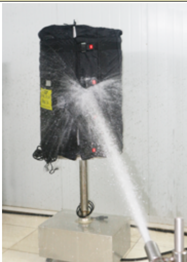
IPx6 testing of jacket heaters
