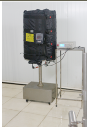
Insulation resistance measurement after IPx6 tests
