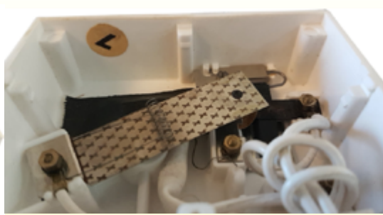
1970 ca. GEC power setting (General Electric, England) on an English heating blanket. Anticipated resistance is clearly visible above the bimetal and slow breaker (Ultimheat Collection).
