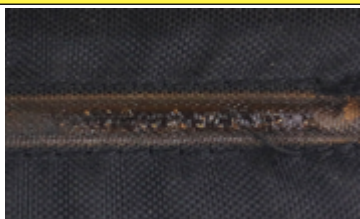
1h at 235°C on the heating cable: The PA66 begins to melt
