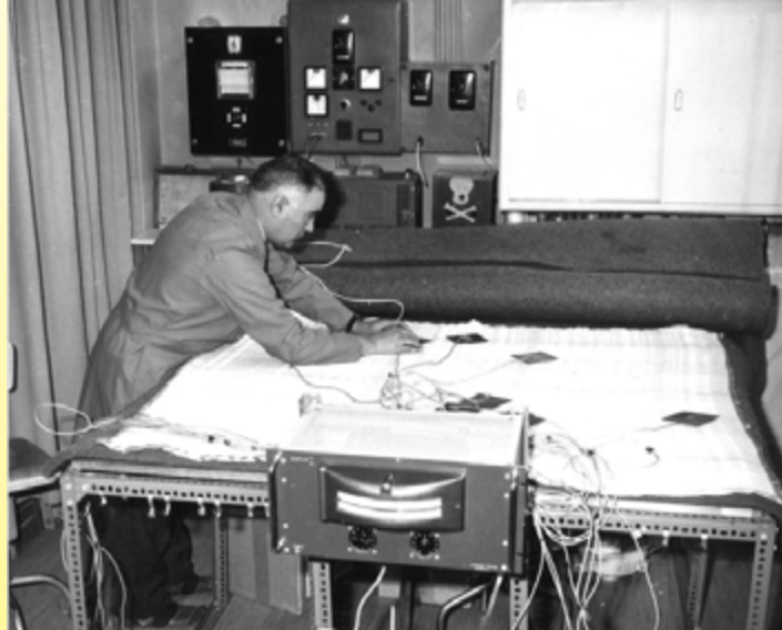
Measuring heated blanket surface temperature (1960 ca, Vedette, Ultiheat Museum)
