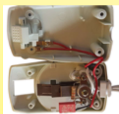
1995: An American power meter heating blanket, similar to that developed more than 50 years earlier by Cook in 1942. Exterior view and view of the internal bimetal has a slow breaker with anticipated resistance. The only notable development in this model is that it includes a noise filter (Collection Ultimheat)
