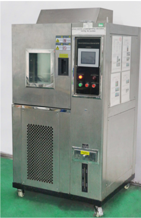
Climate chamber, with temperature adjustment range from -90 to +150^{\circ}C , relative humidity adjustment range 1 to 100%
