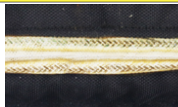
5 minutes at 245°C on the heating cable, the PA66 has melted, and reveals the protective layer of PTFE which is not deteriorated. The protection of the heating cord is always done by PTFE and silicone insulation.
